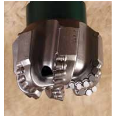
A polycrystalline diamond compact drilling bit used in directional drilling to cut rock. A high fluid flow rate through the bit and diamond tipped cutters ensure high rates of penetration can be achieved with efficient cuttings removal and stable directional performance to drill the well. Photo by J G Domke © http://fwbog.com
