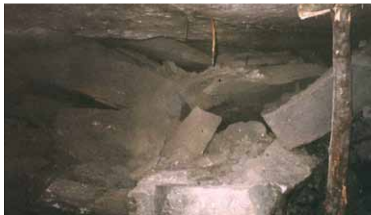
A rare photo showing the formation of goaf after total extraction of a coal seam using longwall methods (Hlobane Colliery, South Africa) © Paul Younger
