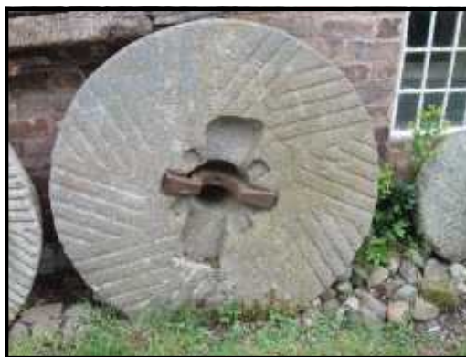
A millstone showing the rhynd and channels
