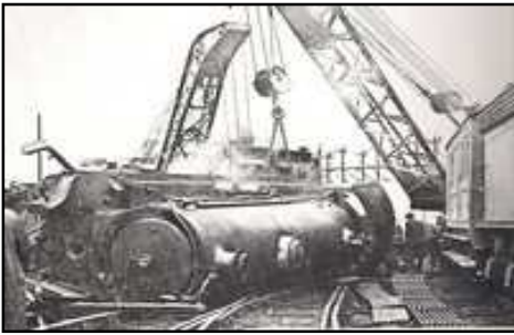
The overturned excursion engine, No. 2164, about to be lifted during the clearing up process.
