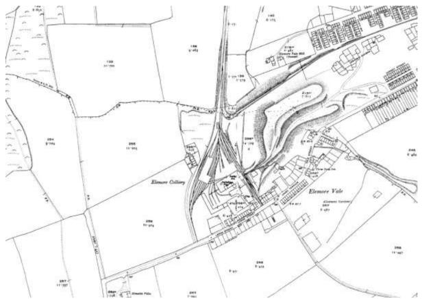
shows an expansion of Railway lines and new Screens/Washing plant and more sidings to the right of the George shaft leading upto the Road, also a new Coal Depot with its own wagon way just north of the present day Pit Baths, also worth noting is the large pit Heap to the East (not in view) which is heading toward the Brickgarth Housing Estate.
